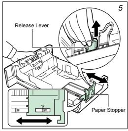
Adjust the position of the paper stopper located at the rear of the paper cassette. Pull the release lever and slide the paper stopper to the desired paper size. When shipped from the factory, the paper cassette is set to A4 size.
