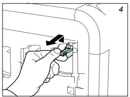
Lift up slightly on the main charger unit and pull it out a short distance as shown in the figure.
