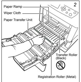
Wipe away the paper dust on the registration roller and the paper ramp using the wiper cloth included in the toner kit.
