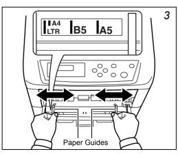
Adjust the position of the paper guides on the MP tray. Standard paper sizes are attached to the MP tray. For standard paper sizes, slide the guides to the position marked correspondingly.
