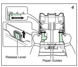
Adjust the position of the paper guides located on the left and right sides of the paper cassette. Pull the release lever on the left side guide and slide to the desired paper size.
