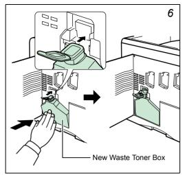
Insert the new waste toner box as shown in the figure. When the box is set correctly, it will snap into place.
