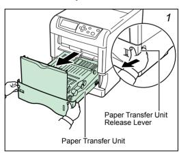
While pulling the green paper transfer unit release lever, pull out the paper transfer unit.
