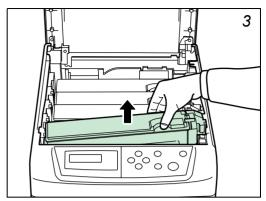
Carefully remove the old toner container from the printer.
