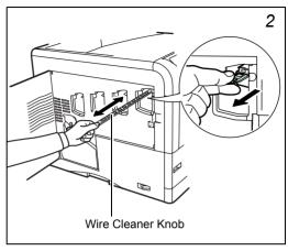
Cleaning the main charger wire — Grasp the tab of the green wire cleaner knob. Gently pull the wire cleaner out and push it back in. Repeat this 2 to 3 times
