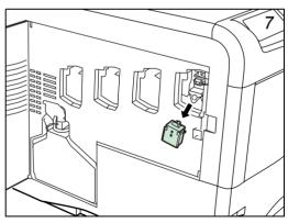
After cleaning is finished, remove the grid cleaner from the printer and discard it. The grid cleaner cannot be reused.
