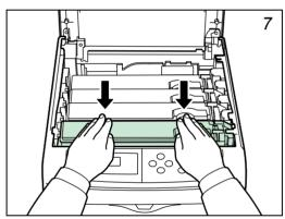
Push down on the top of the toner container to install it firmly in place.
