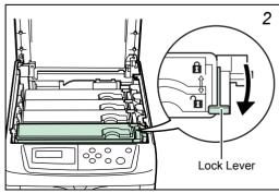
Pull the blue lock lever on the toner container forward towards the unlocked symbol (h).
