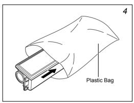
Put the old toner container in the plastic bag (contained in the toner kit) and discard it later according to the local code or regulations for waste disposal.
