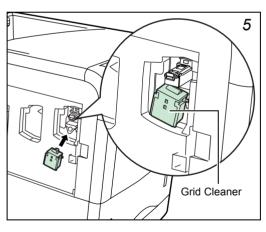
Attach the grid cleaner to the printer with the pad facing up.
