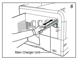
Gently pull the main charger handle out and push it back in. Repeat this 2 to 3 times. These movements clean the grid.
