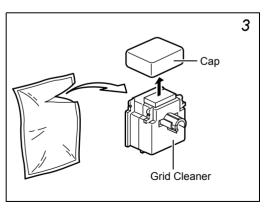
Cleaning the main charger grid — Take the grid cleaner out of the toner kit. Take the grid cleaner out of the protective bag and remove the cap.
