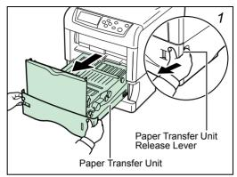
While pulling the green paper transfer unit release lever, pull out the paper transfer unit.
