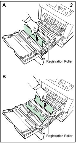
If paper is jammed as shown in **A**, remove the paper by pulling the center up.
