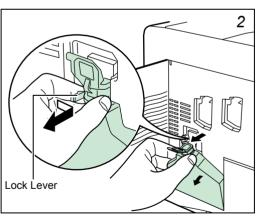
While holding the waste toner box, press the lock lever and then gently remove the waste toner box.
