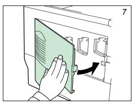
Make sure that the waste toner box is correctly inserted and close the left cover.
