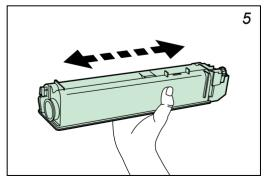
Take the new toner container out of the toner kit. Shake the new toner container 5 or 6 times as shown in the figure in order to distribute the toner evenly inside the container.
