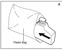
To prevent toner from spilling, put the old waste toner box in the plastic bag (contained in the toner kit) and discard it later according to the local code or regulations for waste disposal.
