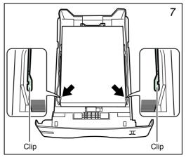
Set the stack of paper so that it is under the clips as shown.
