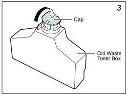
Close the cap to the old waste toner box after removing the box from the printer.
