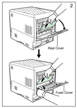
Open the rear cover and then the fuser cover, and remove the jammed paper.
