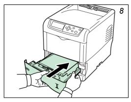
Insert the paper cassette into the slot in the printer. Push it straight in as far as it will go.
